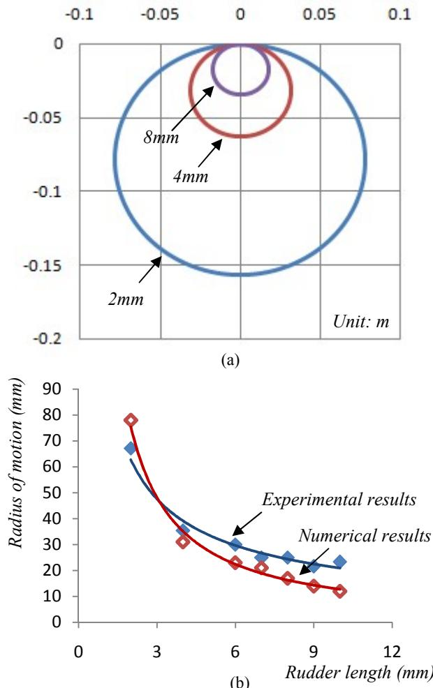
Figure 4: (a) Representative simulated trajectories of 2-, 4-, and 8-mm-long Rudders microboats. (b) The comparison between the simulated results and experimental results of radius of motion vs. rudder length.
