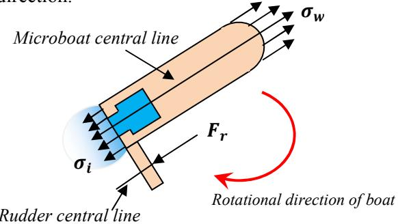
Figure 1: Force analysis of a microboat.  $\sigma_w$  and  $\sigma_i$  are surface tensions before and after the boat, respectively, and  $F_r$  is water resistance on the side rudder.
