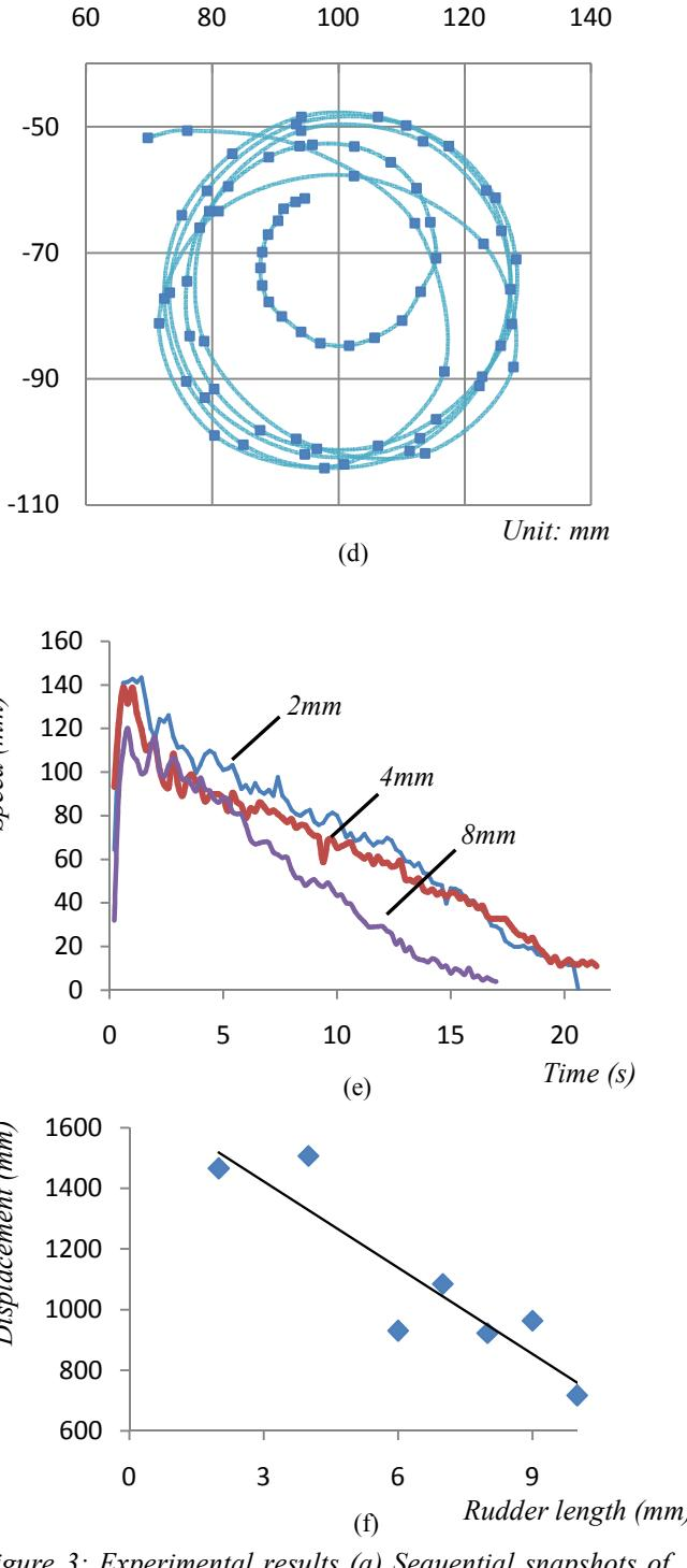
Figure 3: Experimental results (a) Sequential snapshots of a radial motion for the microboat with a 2-mm-long rudder, experimental trajectories for the microboats with (b) 2-, (c) 4-, (d) 8-mm-long rudders, (e) representative speed vs. time curves and (f) total displacement vs. rudder length.
